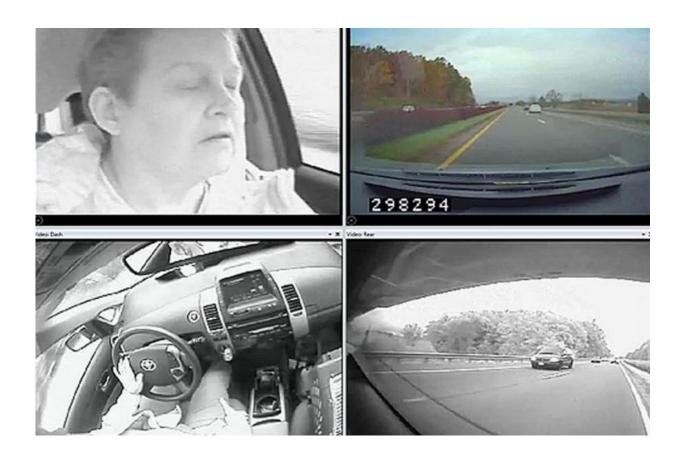
The Virginia Tech Transportation Institute naturalistic driving study method involves equipping vehicles with unobtrusive instrumentation, including an advanced suite of radars, sensors, and cameras -- depicted here with an institute researcher volunteer behind the wheel. The method continuously collects real-world driver performance and behavior. Credit: Virginia Tech
