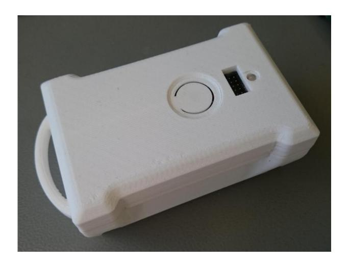
The newly developed fall detector registers falls by comparing pressure changes between a sensor attached to the user's upper body and others installed at various points around the house. Credit: SINTEF
