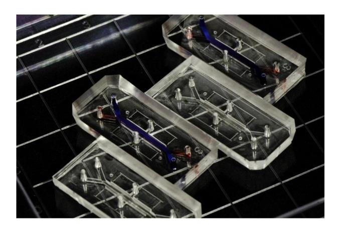
Organs-on-chips, crystal clear, flexible polymers about the size of a computer memory stick that contain hollow channels fabricated using computer microchip manufacturing techniques. These channels are lined by living cells and tissues that mimic organ-level physiology. Credit: Wyss Institute at Harvard University
