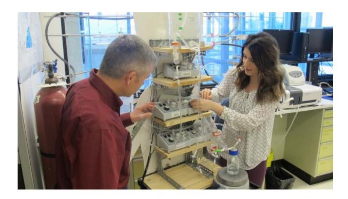
Inspired by a very simplistic model he had read about, Holt, along with master's student Ines Zuna, set out to create the device he envisioned. Six months later, ADAM was born. The completed apparatus accurately demonstrates in a quantitative manner how drugs move through the body by simulating multiple physiological processes, such as how the kidney, liver and heart affect drug distribution and absorption.
