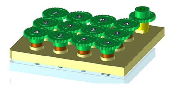
Spin $\Omega$  bio-reactor (top) used to create the conditions for mini-brains to grow. At bottom is a commercially available 12-well lab dish. Credit: Johns Hopkins Medicine
