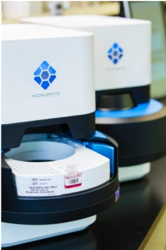
Automated Digital Microscope – Microbes are extracted from a specimen. The extracts are imaged over time using the Automated Digital Microscope to monitor growth under a variety of conditions. The images are processed and microbe identity and antimicrobial susceptibility profiles are reported.
