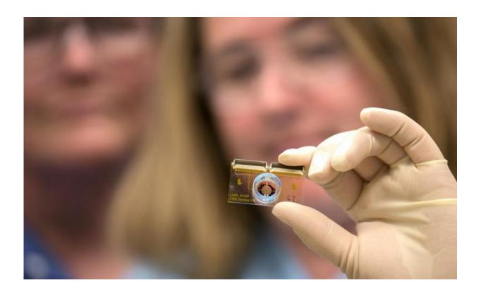
A team of scientists and engineers at Lawrence Livermore National Laboratory is developing "human-on-a-chip," a miniature external replication of the human body, integrating biology and engineering with a combination of microfluidics and multi-electrode arrays. Credit: Julie Russell/LLNL
