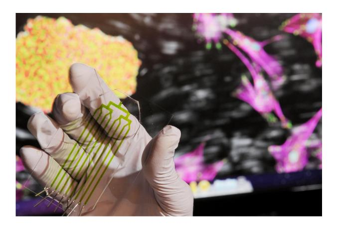
Image shows a close-up view of a microfluidic device that exploits the differences in adhesion strength between derived stem cells and contaminating cell types in a heterogeneous culture to selectively isolate cells of interest using fluid shear forces. Georgia Tech researchers designed the technique to separate the cells. Credit: Gary Meek
