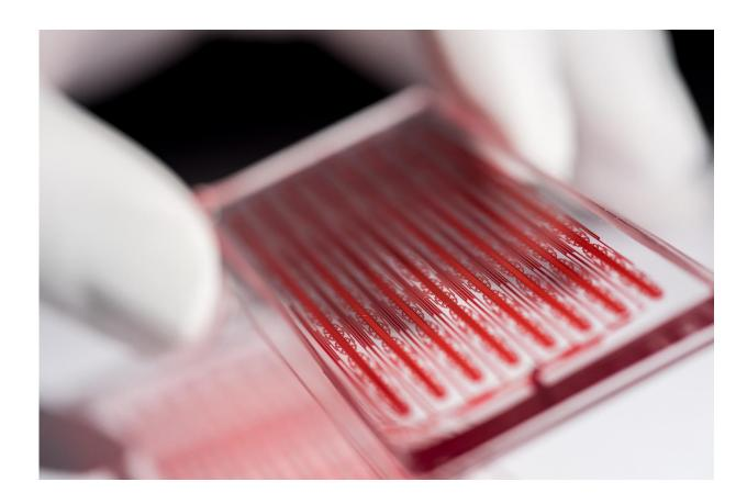
Close-up image shows the microfluidic device used by Georgia Tech researchers to capture cancer cell clusters in blood samples. The fluid shown in the device is a colored liquid designed to simulate the appearance of blood. Credit: Rob Felt,
