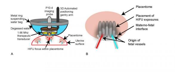
Diagram of side view of equipment setup and high-intensity focused ultrasound (HIFU) exposure placement. (A) Setup of the ring-shaped HIFU transducer and central diagnostic ultrasound probe within a bag of degassed water. (B) Placement of HIFU lesions in a linear track across the origin of the fetal vessels. Credit: Shawi et al. / *Science Translational Medicine* (2016)
