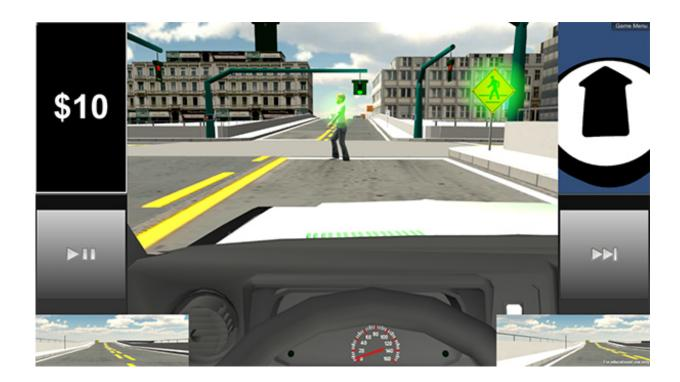
When the driver fails to look at critical elements in the virtual surroundings, then the simulator will stop and highlight the critical objects. Credit: Robotics and Autonomous Systems Lab/Vanderbilt University
