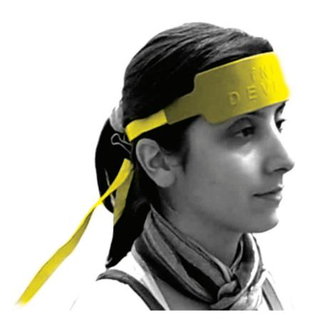
The fNIR sensor, which is placed around the forehead like a headband, uses LEDs that shine near-infrared light to sample from 16 brain areas. Researchers use the technology to monitor oxygenation in the brain while the subject performs cognitive tasks. Credit: Drexel University
