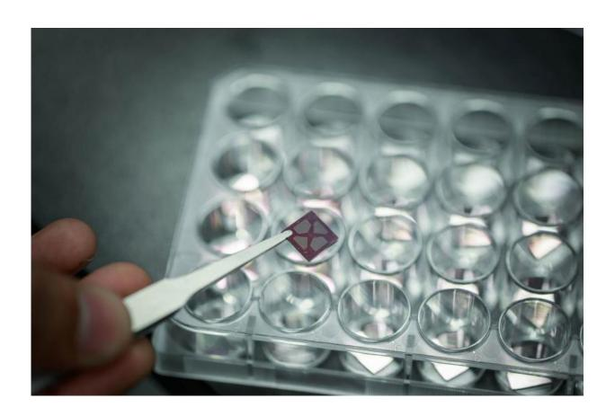
The core material used for the new immunosensor that detects proteins in the blood stream following a heart attack, providing results in just 1 minute. Credit: UNIST
