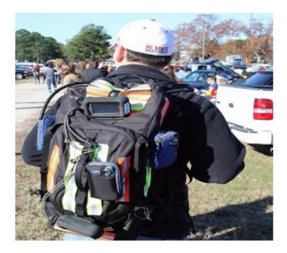
Before, during and after football games, a small team of researchers carried the mobile air monitor in a backpack equipped with GPS location devices. Video cameras collected visual data that allowed researchers to identify sources of any recorded increases in emissions. Credit: North Carolina State University
