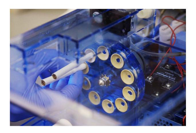
In a published study, the Wyss Institute describes an instrument they engineered that can "breathe" in and out, actively smoke regular and electronic cigarettes much like a human. Individual mouth pieces in a rotating unit of the smoking machine are fitted with standard cigarettes. Credit: Wyss Institute at Harvard University
