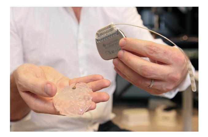
The brain-spine interface uses a brain implant like this one to detect spiking activity in the brain's motor cortex. Seen here, a microelectrode array and a silicon model of a primate's brain, as well as a pulse generator used to stimulate electrodes implanted on the spinal cord. Credit: Alain Herzog / EPFL
