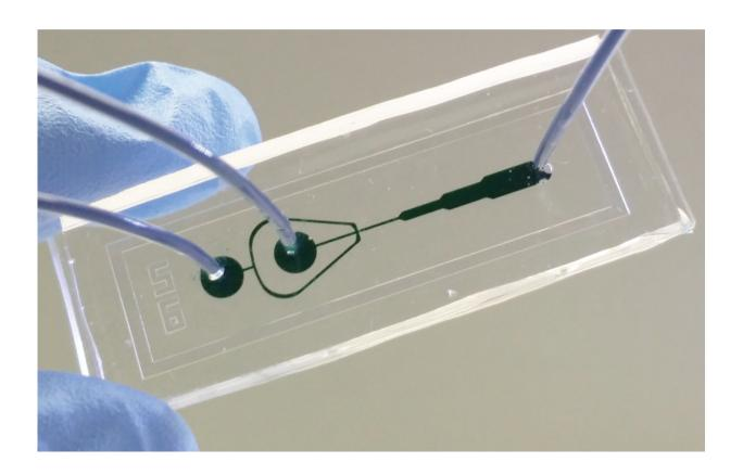
UGA researchers encapsulated individual *Neurospora crassa* cells in droplets using this new microfluidics device. (The channel is dyed green.) The device allowed them to track tens of thousands of cells with single-cell precision as they studied the cells' circadian rhythms. Credit: UGA
