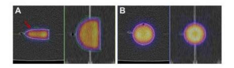
SPECT/CT reconstructions and VOIs used for determination of calibration factors for the adult kidney filled with Lu-177 (A) and the corresponding sphere filled with I-131 (B). Credit: University of Würzburg
