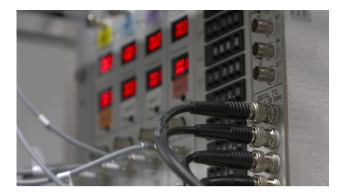
Preamplifiers and amplifiers used for the in vivo recording experiments described in the study. Credit: MotionManager
