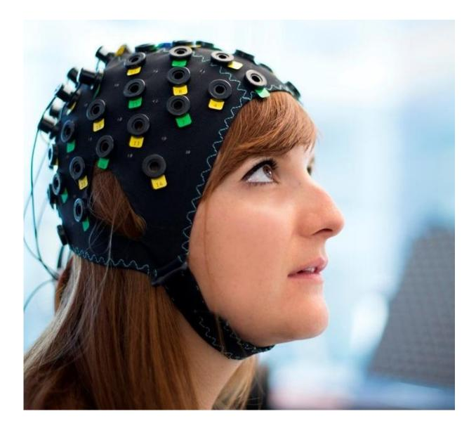
NIRS/EEG brain computer interface system shown on a model. Credit: Wyss
