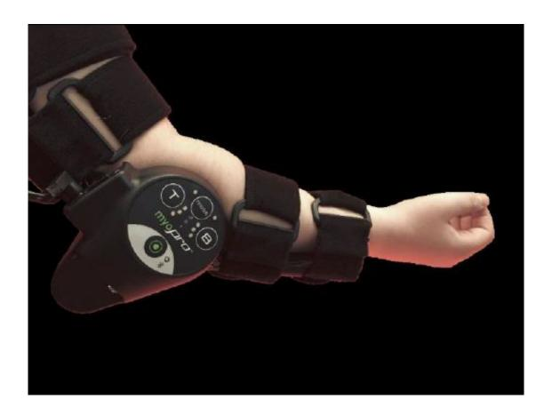
This powered orthotic arm brace, called a MyoPro device, amplifies weak muscle signals in a patient's arm. Credit: Myomo, Inc.
