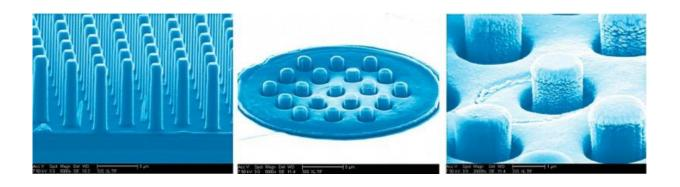
Scanning electron micrograph (SEM) image of individual nanowires and groupies of nanowires. Each wire can produce an electric current when hit by light. Credit: University of California - San Diego
