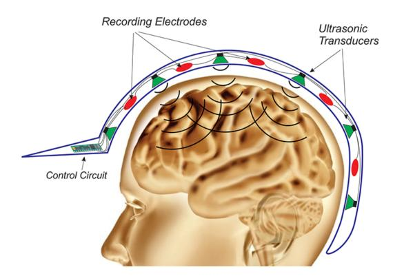
This wearable device would noninvasively stop the progression of seizure activity in the brain by launching a random spatio-temporal pattern of ultrasonic waves from outside of the brain to target populations of neurons in various locations across the cortex to stop the seizure propagation in its tracks. Credit: Carnegie Mellon University Department of Electrical and Computer Engineering
