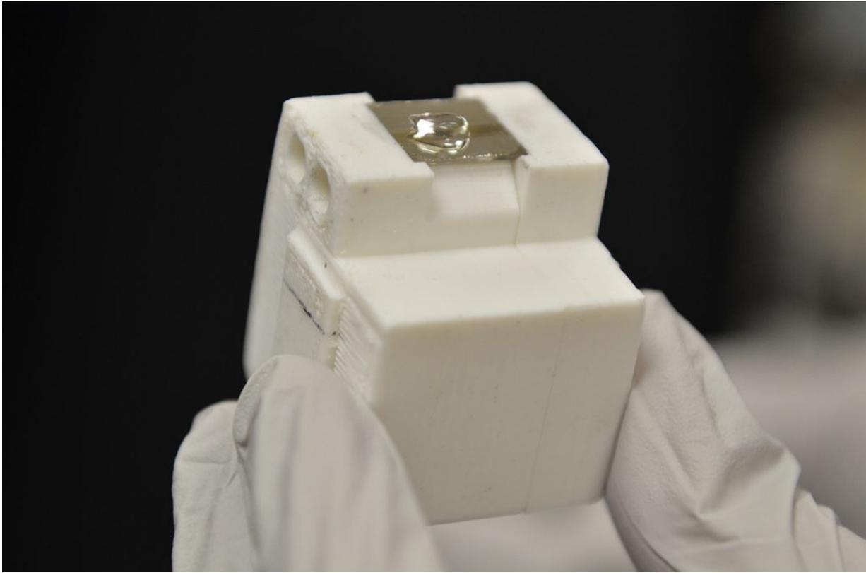
A close-up of the specialized waveguide that helps deliver laser light with higher accuracy, efficacy and safety than its predecessors. Credit: Stephen Schmidt, CAFNR
