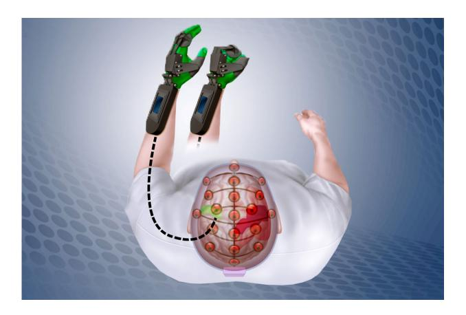
The Ipsihand detects electrical signals in the uninjured part of the brain (green), and opens and closes a plastic brace fitted onto the paralyzed hand (green). By doing so, it helps train the uninjured brain areas to take over functions previously performed by injured areas (red). Credit: Matthew Holt/Sara Moser
