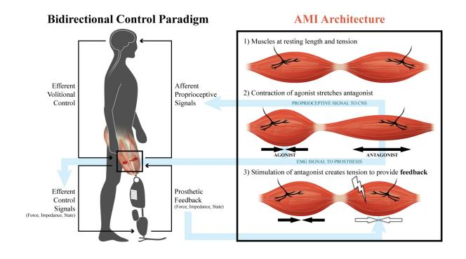
The agonist-antagonist myoplastic interface (AMI) is an advanced neural interfacing construct for amputation surgeries to enable robust bidirectional communication with prostheses and provide naturally-generated sensory feedback information to the user. Credit: Stephanie Ku
