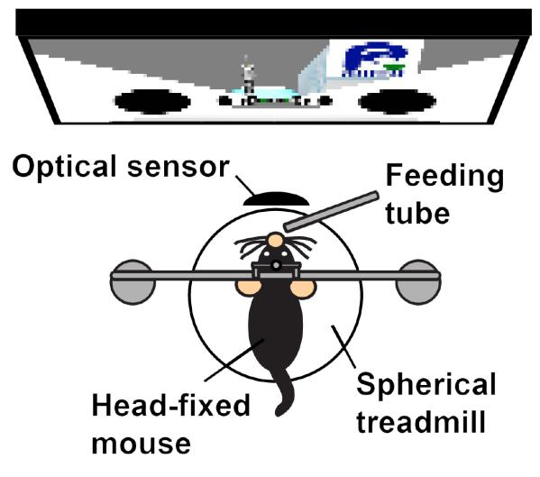
A mouse sat on a spherical treadmill and the rotation was detected by an optical motion sensor. The signal was fed to a program that renders VR scenes as visual feedback on a wide LCD monitor placed in front of the mouse. Credit: RIKEN
