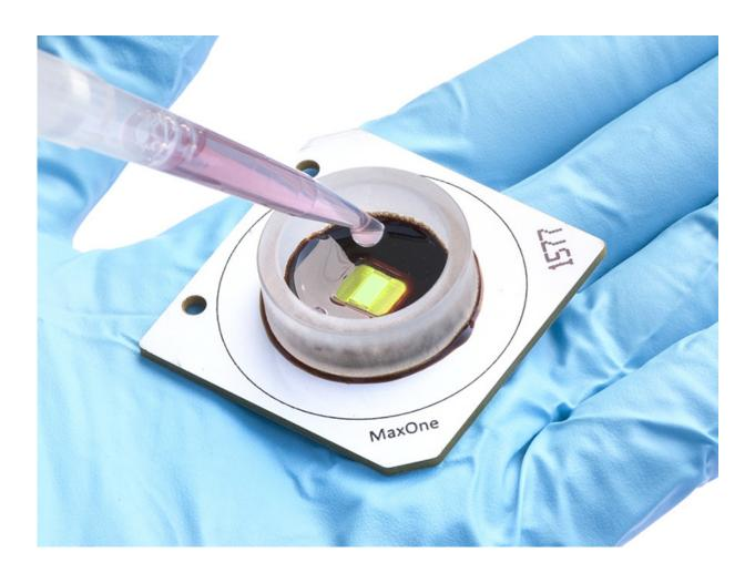
"MaxOne," the microelectrode platform for electrophysiological cell analysis. Credit: MaxWell Biosystems AG
