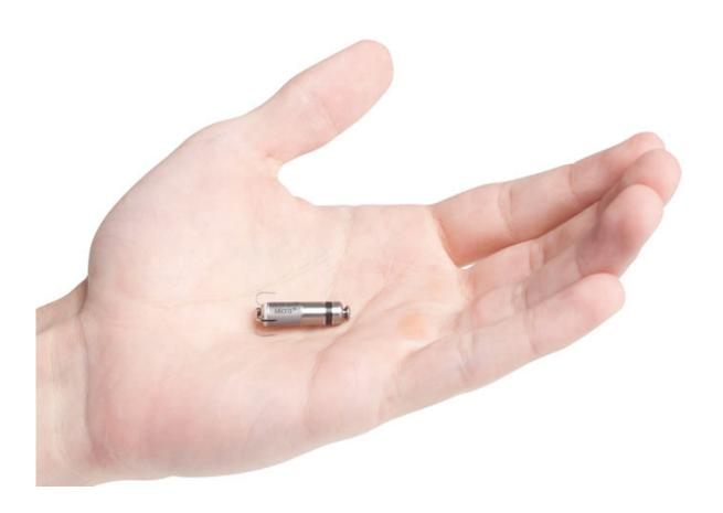
The Micra Transcatheter Pacing System is one-tenth the size of conventional pacemakers. Credit: Medtronic
