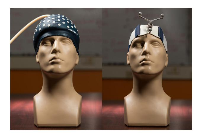
The granular-jamming cap, left, compared to the current elastic headband that allows the computer to track the position of a patient's head during endonasal surgery. Credit: Joe Howell, Vanderbilt University
