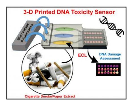
Small 3-D printed array created by University of Connecticut chemists quickly detects potential DNA damage from toxic chemicals. Credit: Karteek Kadimisetty and the journal *ACS Sensors*.
