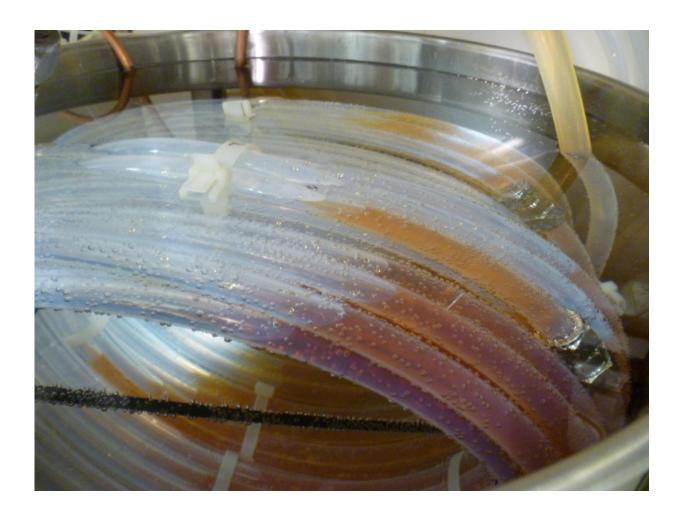
Photograph of deprotection gas/liquid reactor during processing. Credit: Eli Lilly and Company.
