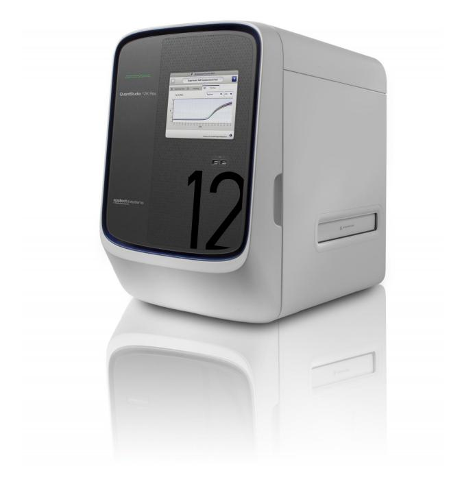
The QuantStudio 12 is the Thermo Fisher Scientific instrument that processes the OpenArray plates that carry the PCR reagents and the nucleic acid samples accomplishing the multiplex pathogen detection. Note: This OpenArray Platform is a research use only device and is not cleared or approved for clinical use.
