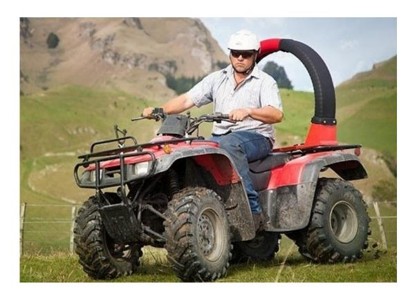
Rider wearing Quad bike helmet with Lifeguard Operator Protective Devices attached to bike. Credit: UNSW
