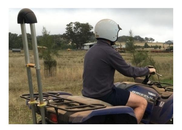
Rider wearing a Quad bike helmet with Quadbar Operator Protective Device attached to bike. Credit: UNSW
