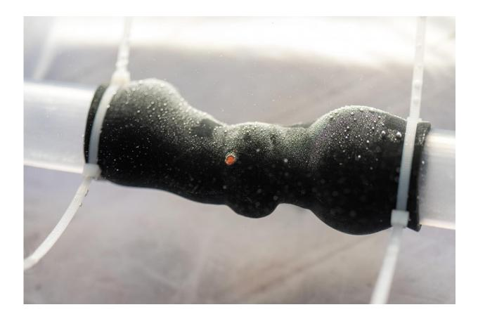
New 3-D printing technologies allow researchers to create patient-specific heart valve models that mimic the physiological qualities of the real valves. This image shows the submerged valve during flow testing. Credit: Rob Felt
