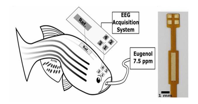
Schematic illustration of long-term precise EEG measurement method and electrodes to measure EEG in zebrafish, developed by Sohee Kim's research team. Credit: DGIST
