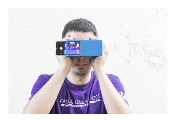
BiliScreen is a new smartphone app that can screen for pancreatic cancer by having users snap a selfie. It's shown here with a 3-D printed box that helps control lighting conditions to detect signs of jaundice in a person's eye. Credit: Dennis Wise/University of Washington
