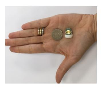
The TaiNi device (pictured next to the 20 pence piece) is smaller and lighter compared to conventional sensor technology. Credit: Imperial College London
