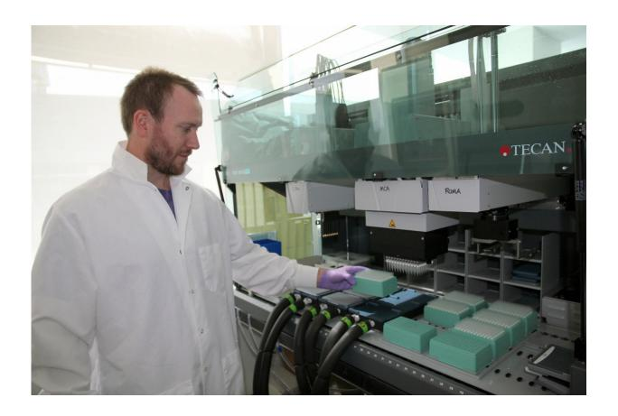
Brian Thompson, a research associate in the Single Cell Genomics Center at Bigelow Laboratory for Ocean Sciences, loads samples into a liquid handling robot. The Laboratory recently published the details of significant advances in single cell genomics technology, which allows scientists to study the genes of individual cells. Credit: Bigelow Laboratory
