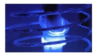
Thermal image showing that the alternating magnetic fields selectively heat the metal knee joint. Credit: UT Southwestern
