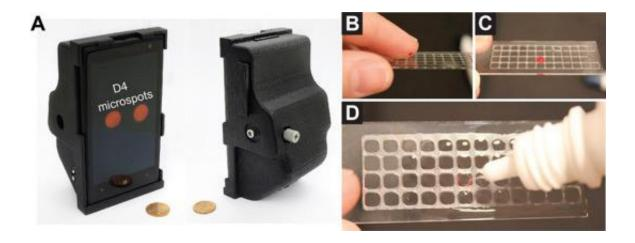
The photo on the left shows the 3-D printed smartphone attachment that uses the phone's camera to review the results of the assay. The photo series on the right shows the process to administer a blood sample onto the D4 assay. Credit: Daniel Joh, Duke University
