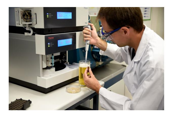
FAU-based researcher Thomas Sommer preparing a sample of beer. After processing, the level of hordenine in the sample is determined using high-performance liquid chromatography and mass spectrometry. Credit: FAU/Katharina Götz
