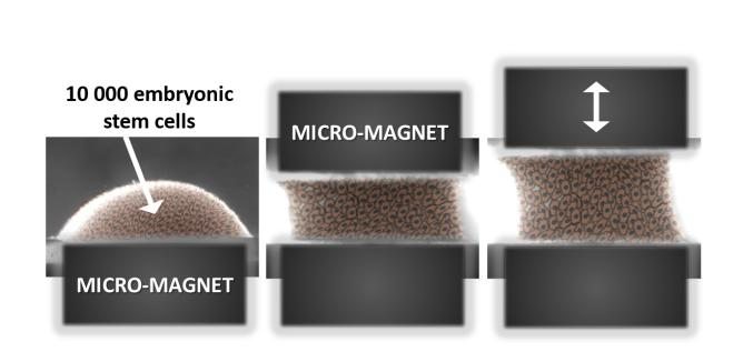
The magnetic stretcher: this all-in-one system can both form and mechanically stimulate an aggregate of embryonic stem cells. The two micromagnets, one of which is mobile, frame the resulting embryonic body, and cyclical stimulation can be adapted to the type of tissue being sought. Credit: Claire Wilhelm / Laboratoire Matière et systèmes complexes (CNRS/Université Paris Diderot).
