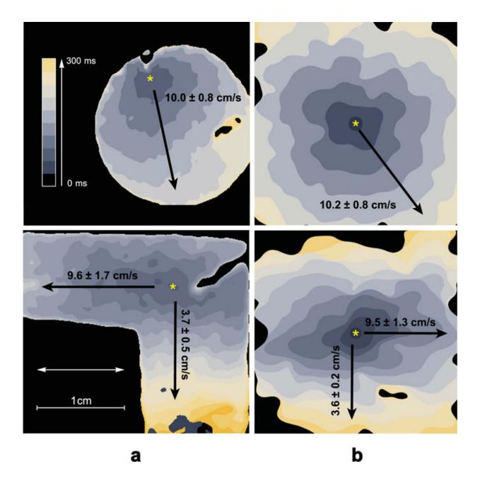
Electrical wave propagation in isotropic (upper row) and anisotropic samples (lower row): a)Experimental samples, b)Simulation. Credit: 10.1038/s41598-017-07653-3
