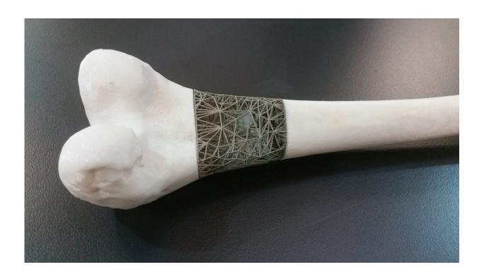
3-D-printed element inserted into bone. Credit: RMIT University
