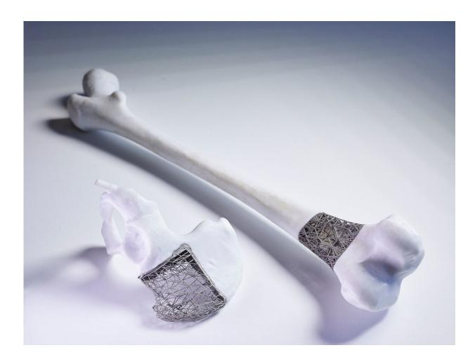
3-D-printed element inserted into bone, with additional examples. Credit: RMIT University
