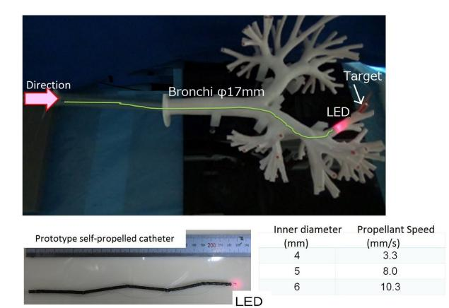
Delivery experiment within bronchus model and a self-propelled catheter prototype. Credit: Hideyuki Tsukagoshi
