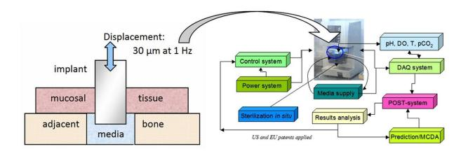
Benchtop test setup for the high-output screening of dental implants (DO = dissolved oxygen, T = temperature, pCO2 = partial pressure of CO2, DAQ = data acquisition, POST = post-processing data treatment, MCDA = multi-criteria decision aiding). Credit: National Institute for Materials Science
