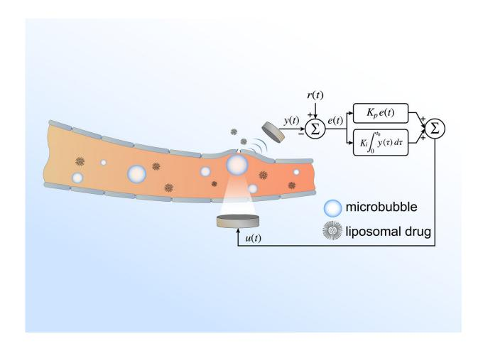
Representation of the drug delivery system. Serving as the acoustic indicator of drug delivery dosage, the microbubble emission signal y(t) is used to find the expected controller output u(f) which is fed back to help control ultrasound transducer transmission. Credit: Tao Sun, Brigham and Women's Hospital
