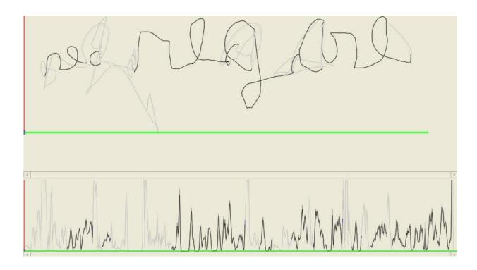
Black lines show what the child actually wrote on the page; grey lines, recorded by the tablet, show in-air movements when the child paused. This example shows that the child started to write; stopped, then continued. The result is an irregularly produced word which presents a spelling mistake at the end. Below: Evolution in speed over time. Grey lines show in-air movements recorded by the tablet. Credit: © Sonia Kandel for GIPSA-Lab (CNRS/Université Grenoble Alpes/Grenoble INP).
