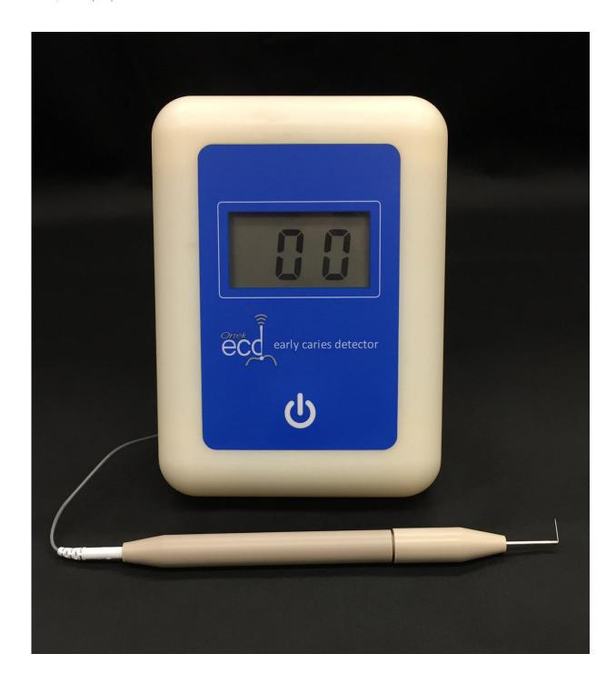
The Electronic Cavity Detection (ECD) System is a battery-powered device that may help dentists detect early signs of cavities well before tooth decay is revealed by X-rays. Credit: Stony Brook University
