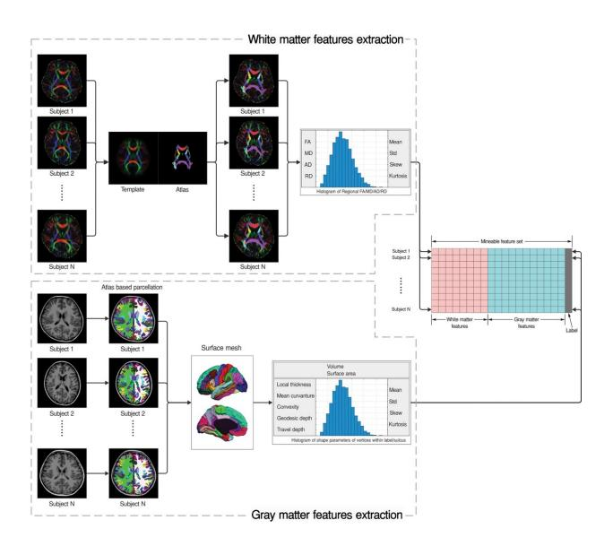
Diagram shows the workflow for extracting radiomics features from T1-weighted and diffusion-tensor images. FA = fractional anisotropy, MD =
