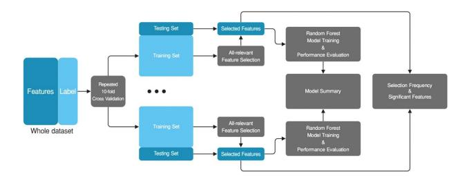
This flowchart shows feature selection and model training. Rectangles in blue represent data and rectangles in gray represent the processes. The all-relevant features selection step was nested in repeated 10-fold cross validation. Credit: Radiological Society of North America
